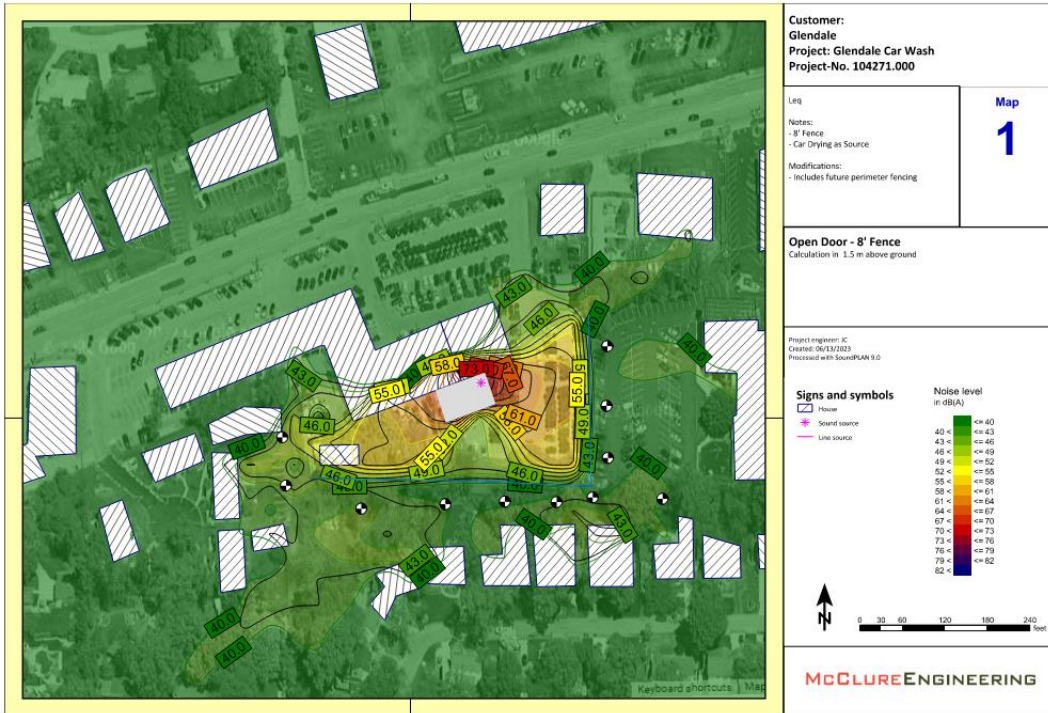
Figure 4 – Sound Map of Carwash Doors Open (8' fence at PL)– No Background Sound
